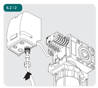
Feed the cables through the screw fitting into the operator.
